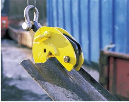
The PP pile pulling clamps are designed to pull out driven piles or trench shielding. The clamps have a narrow opening and a deep slot to ensure that the pile is gripped firmly. It is extremely difficult to determine the forces required to pull out driven piles so it is recommended that a load indicator is used to ensure the WLL of the clamp is not exceeded.
