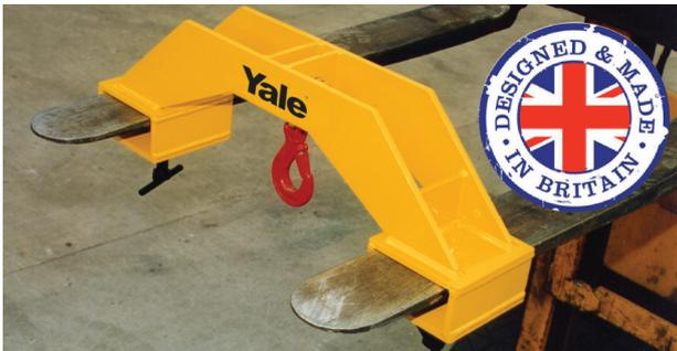
The FLTH tine hook is designed to convert your forklift truck into a crane. This is done by simply sliding the FLTH over the tines of your forklift truck. The FLTH is fastened to the tines by tightening the two threaded bars underneath each tine. The unit is supplied a standard with a swivel safety hook.
