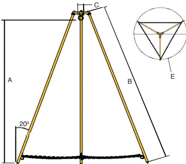
The Camlok Shearlegs have been designed to be simple and easy to erect and operate. Each set of shearlegs are supplied, as standard, fitted with safety chains and a large eyebolt for the suspension of hand operated lifting mechanisms, chain blocks or pulleys.
