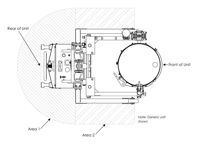
WARNING - DO NOT STAND UNDERNEATH A RAISED LOAD, WITHIN THE CONFINES OF THE UNIT OR IN FRONT OF THE UNIT DURING OPERATION.
