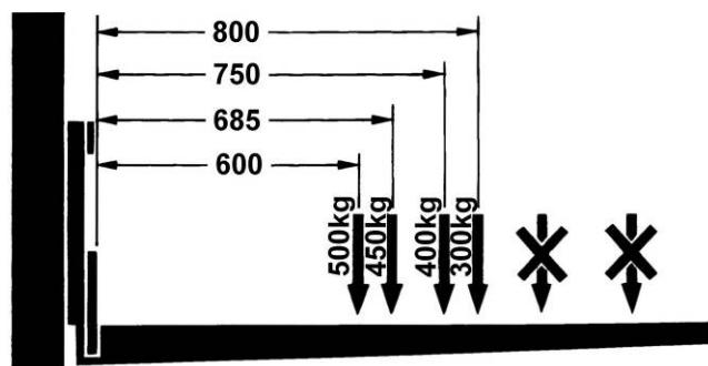
The load must equally balanced on both forks
