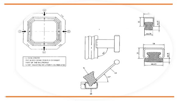
Badly Worn or damaged seals should be re-placed prior to use. New seals can be inserted into seal profile using insert bar at an angle of 45 Deg, see diagram above.
