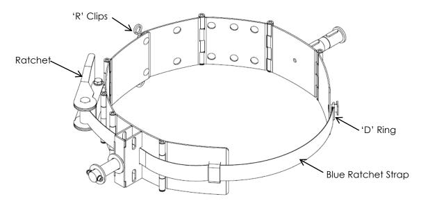
• Hook the 'D' ring that is on the end of the blue ratchet strap onto the securing pin, which is on the last band section on the left hand arm and pull on the tail of the blue ratchet strap to take out the slack. Then use the ratchet to tension the clamping band, this should be tightened until the drum starts to show signs of deflection.
