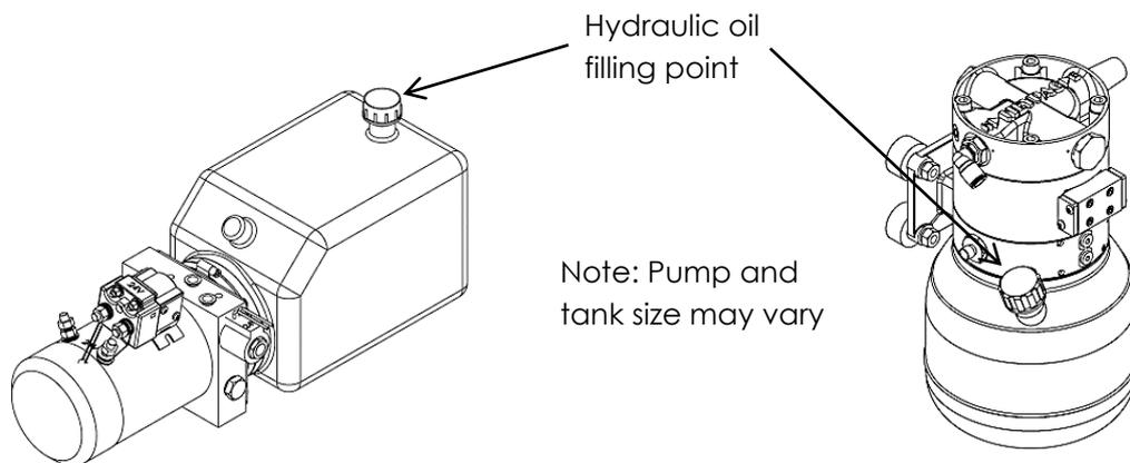
When replacing oil, fill oil to the line or to the middle of the sight glass. Operate all unit functions to their full extents. Return unit head to its lowest position and recheck the oil level, top up if required.
