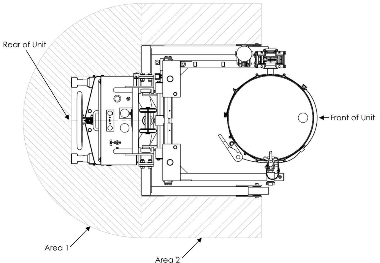
**WARNING - DO NOT STAND UNDERNEATH A RAISED LOAD, WITHIN THE CONFINES OF THE UNIT OR IN FRONT OF THE UNIT DURING OPERATION.**
