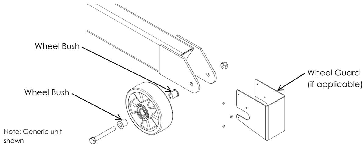
To replace the rear wheels, ensure that the head of the unit is in its lowest position. Place a wooden block or equivalent under the rear wheel legs, behind the steering mechanism, and jack up both wheels centrally under the unit by 150mm. Unbolt each wheel using two 19mm spanners. Replace the wheels ensuring that the wheel bushes are re-fitted into the wheels prior to re-bolting.
