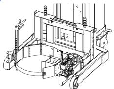
secure a drum. The adaptor should only be used to pick up small drums that do not fit in the normal head arrangement.
