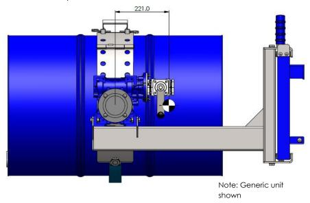
WARNING - ROTATING A DRUM WITH A HIGHER OFFSET LOAD IS TREATED AS MISUSE AND MAY DAMAGE THE UNIT.
