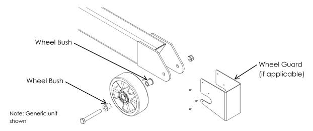
To replace the rear wheels, ensure that the head of the unit is in its lowest position. Place a wooden block or equivalent under the rear wheel legs, behind the steering mechanism, and jack up both wheels centrally under the unit by 150mm. Unbolt each wheel using two 19mm spanners. Replace the wheels ensuring that the wheel bushes are re-fitted into the wheels prior to re-bolting.
