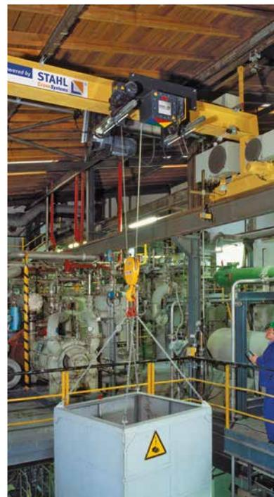
An explosion-protected SH Ex wire rope hoist transports goods through a shaft over several storeys of a chemical plant. The single-girder overhead travelling crane with a load capacity of 5,000 kg is operated by radio remote control.
