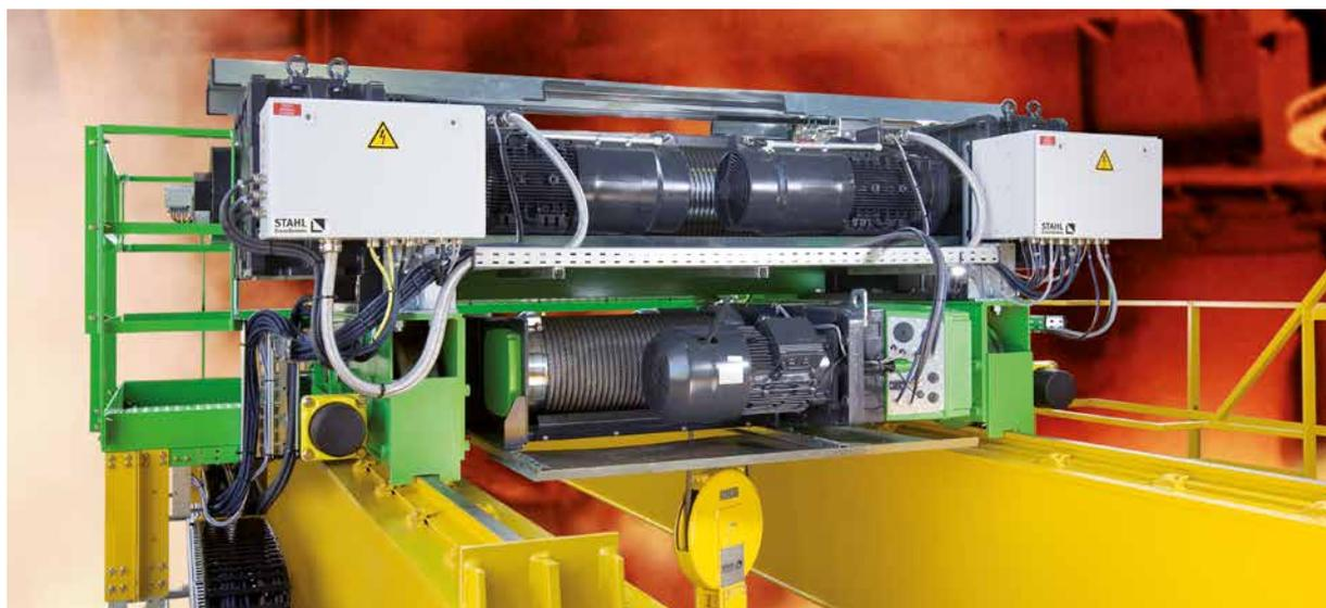
Unit with an SH wire rope hoist as auxiliary hoist
